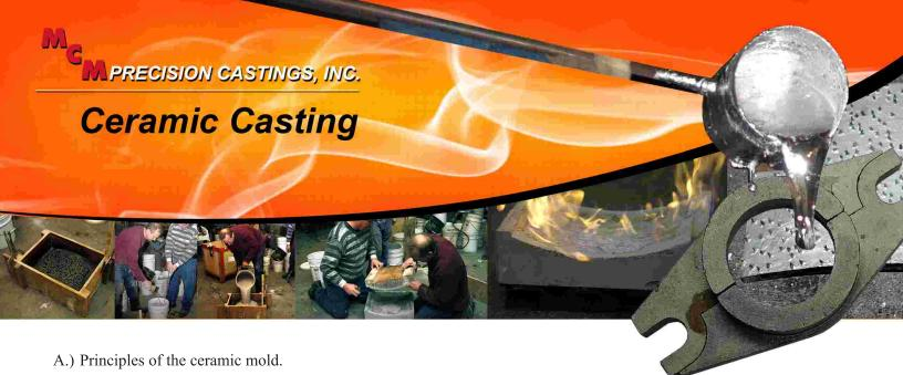
The ceramic mold process is a method of mold making and precision casting using conventional patterns with no size restrictions.
